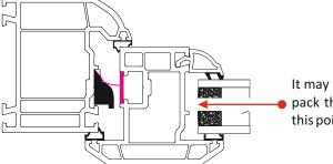
It may be necessary to pack the sash/glass at this point as shown
