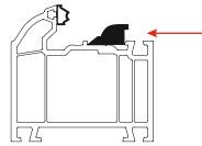
Fit a 13mm Frame Wedge to the outer frame on the stay fixing area
